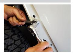
Place the fender back into place, and attach using an M6 bolt, lock washer and flat washer.
